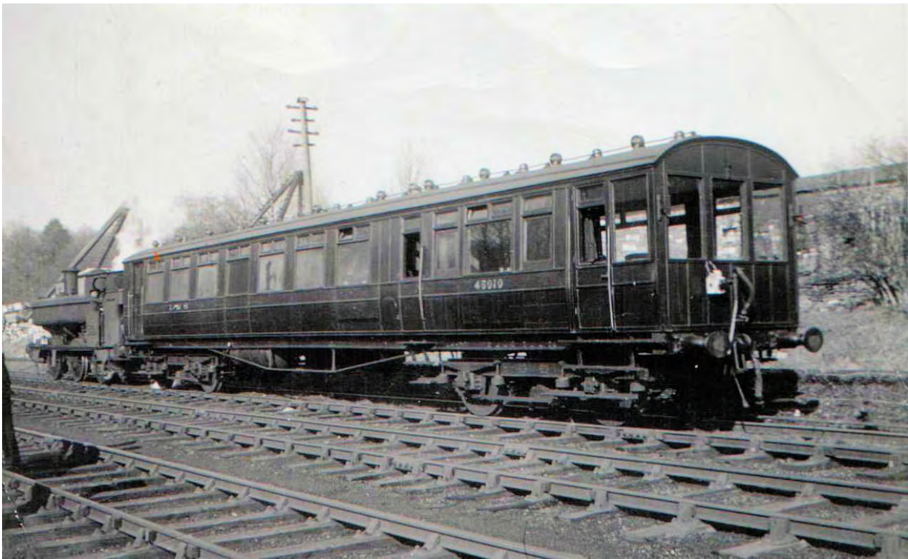
The Crewe District Signal and Telegraph Engineers coach LMS 45010 seen here hauled by GWR '2021' class tank at Bicslade Wharf on a GWR/LMS joint line. The coach was used for many tours of inspection on the Crewe S&T Division. It had an observation compartment at one end equipped with chairs and tables and could be used as a dining room. In the centre were compartments including a kitchen with a gas cooker and sink, a toilet and bath and also a bedroom. The other end was fitted as an office with desks and cupboards, It had been made for J. Follows, late superintendent of the Midland Railway.
