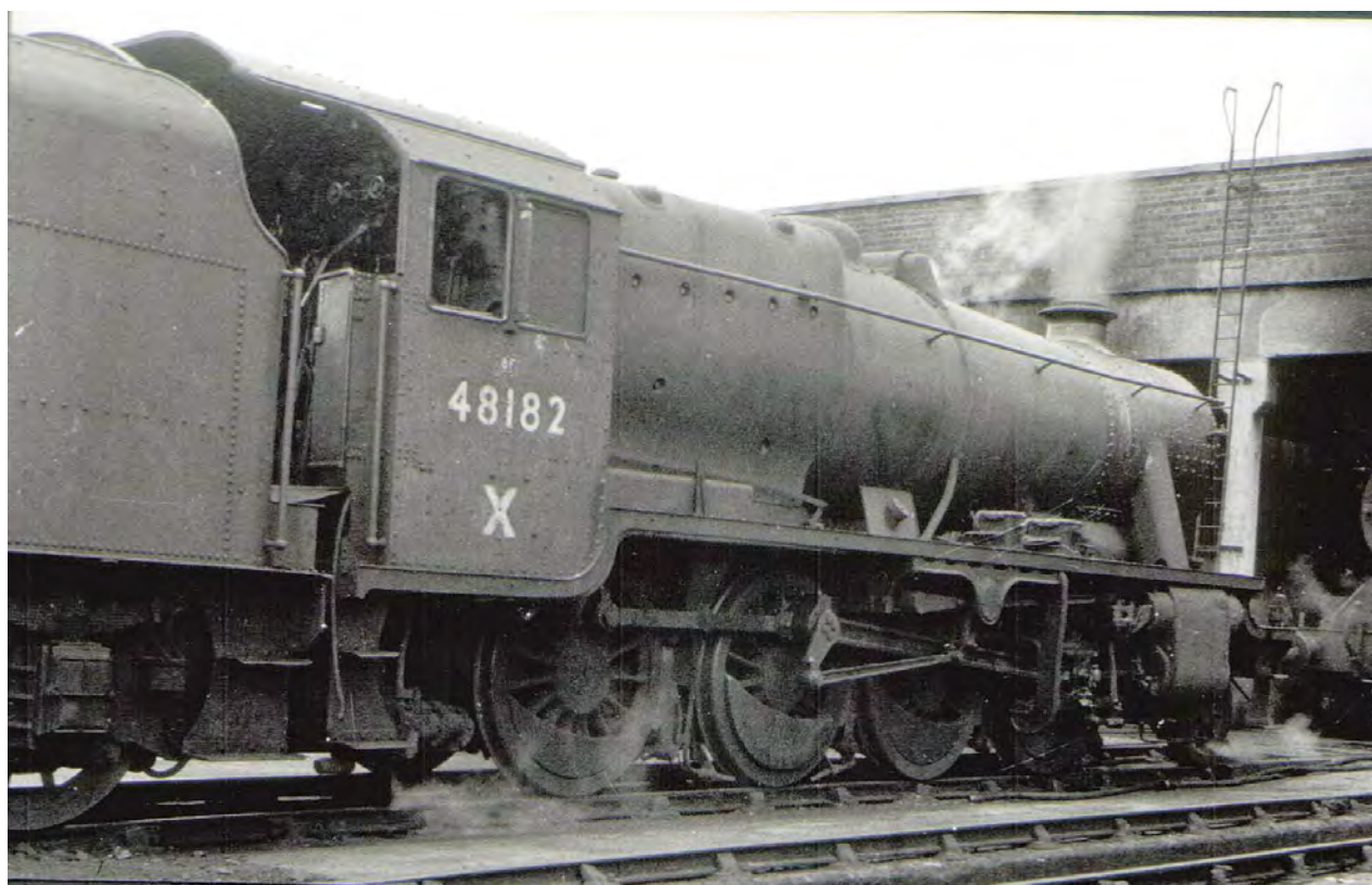
Plate 8 - One of the fifty 8Fs taking part in the experimental fitting of manual blow down or de-sludging valves seen here on Aston shed c.1950-2.
